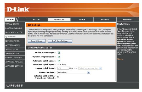
Manual Uplink The speed at which data can be transferred from the router to your ISP. This is determined by your ISP. ISP's often speed **Speed:** as a download/upload pair. For example, 1.5Mbits/284Kbits. Using this example, you would enter 284. Alternatively you can test your uplink speed with a service such as www.dslreports.com.
